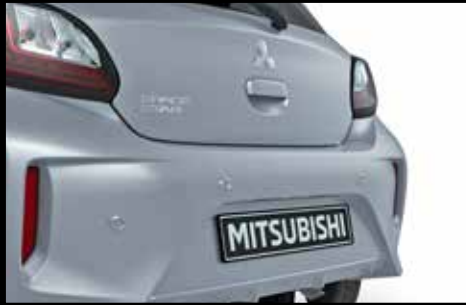
▲ Rear parking assistance 4 sensors. Painted in body colour. For part numbers see quick reference list.
